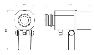
**燈體** ┃ 鋁合金 **支架** ┃ 耐候鋼材 **Luminaire** | Aluminum alloy **Support** | Steel
